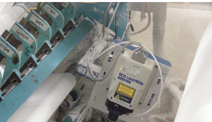
LaserSpeed Pro non-contact laser gauge at slitter/rewinder in sanitary product manufacturing plant.
