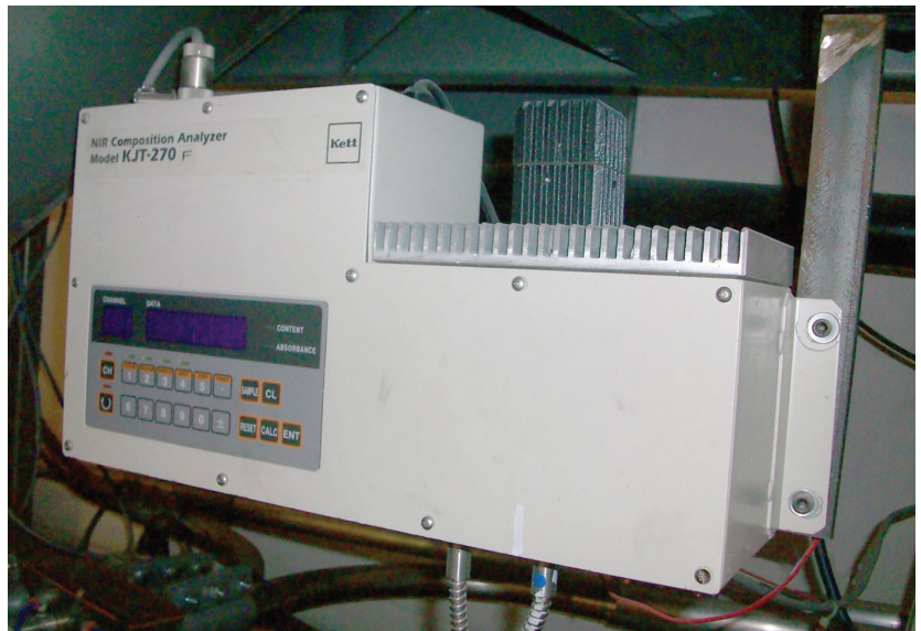
NIR moisture meters allow very accurate instant measurement of solids, liquids, and slurries without contact or sample preparation.
