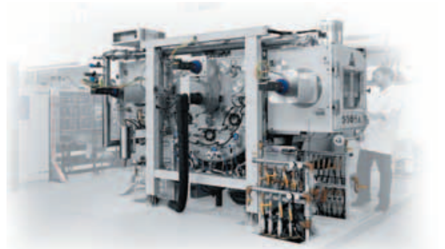
Applied Films' new SmartWeb machine has three deposition chambers. Each has its own pump-down capability.
