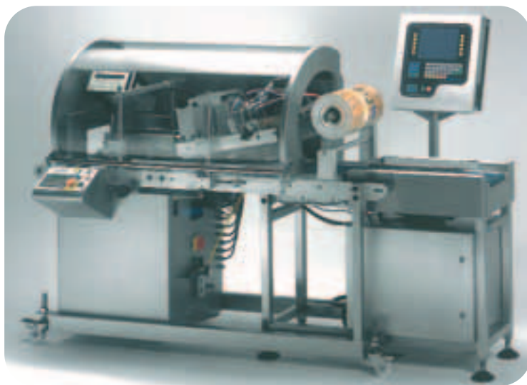
The SE Sleeve labeling/sleeving system from SE Dynarap combines applicator machine and high quality labels/sleeve consumables, which are printed on a quality thin sleeving board.
