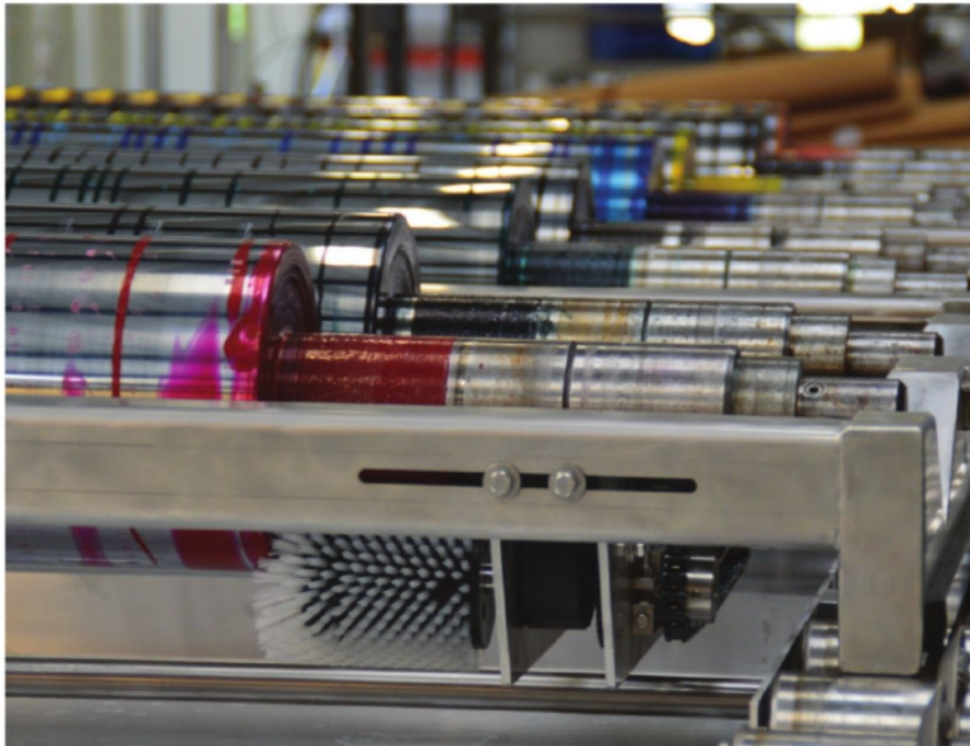
The PLC-controlled machines can be equipped with rotating brushes, which make it possible to clean gravure cylinders in the machine.
