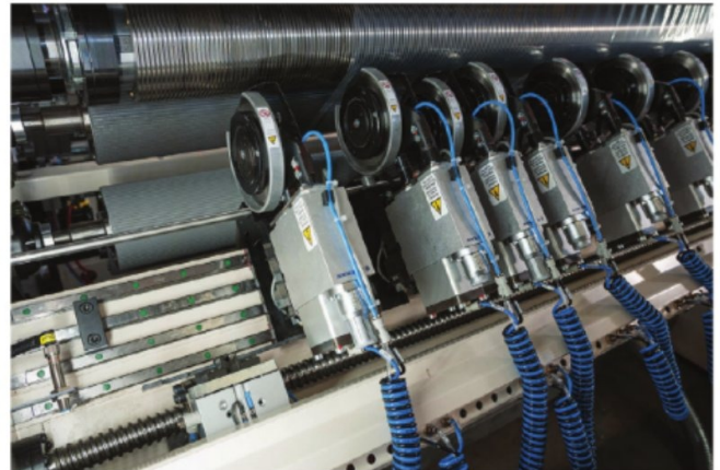
The knife section on LAEM IMS machine FLEXISLIT
